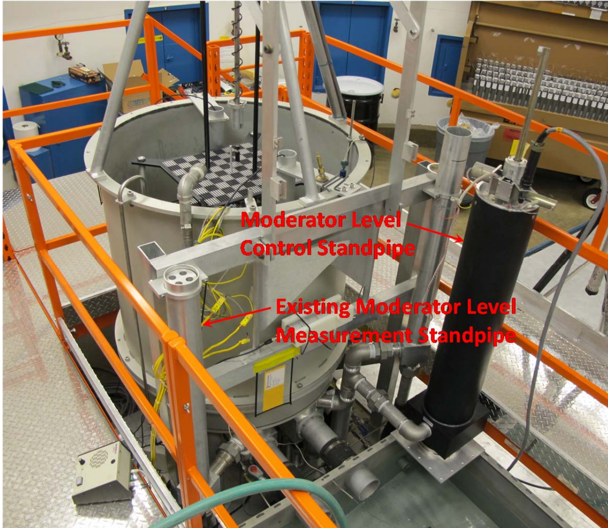
Figure 12. Photograph of the Critical Assembly showing the Moderator Level Control Standpipe and the Moderator Level Measurement Standpipe.
