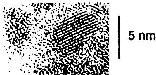
Figure 2. A Transmission electron micrograph of a 4nm GaAs noncrystal on a metal grid.
