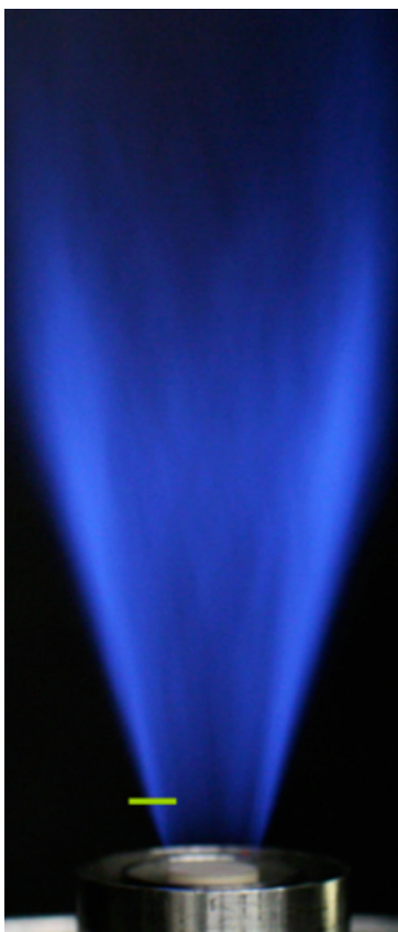
Figure 2-3. Photograph of premixed turbulent flame SwB2 and comparisons of measured results and laminar unstrained 1D Chemkin calculations at \phi = 0.77 .
