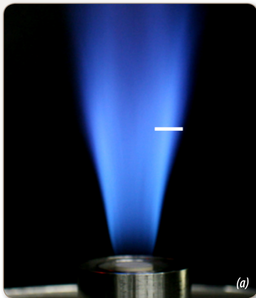
Figure 1-1. Photographs of two highly stratified flames stabilized on the Cambridge burner: (a) nonswirling and (b) swirling. The white line in (a) indicates the region where the flame is burning through the middle of the turbulent mixing layer between two annular streams of different equivalence ratio ( \phi_{inner} = 1.125 , \phi_{outer} = 0.375 ).
