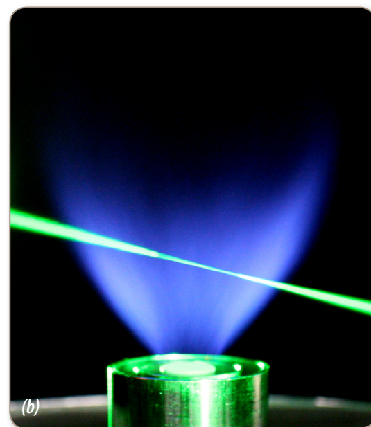
Figure 1-1. Photographs of two highly stratified flames stabilized on the Cambridge burner: (a) nonswirling and (b) swirling. The white line in (a) indicates the region where the flame is burning through the middle of the turbulent mixing layer between two annular streams of different equivalence ratio ( \phi_{inner} = 1.125 , \phi_{outer} = 0.375 ).
