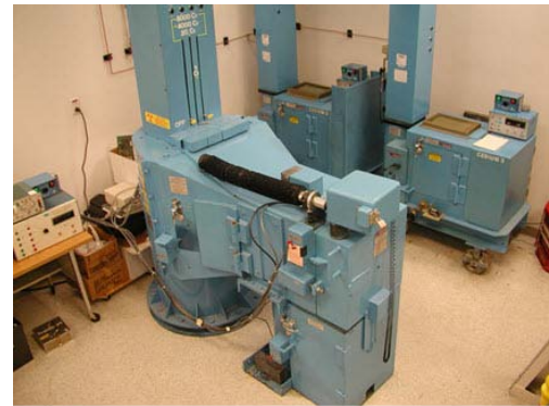
Figure 1. Sandia Radiation Physics Department Shepherd ^{60}\text{Co} and ^{137}\text{Cs} gamma radiation sources.
