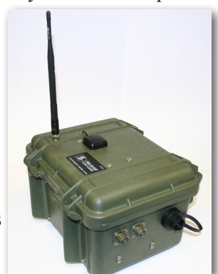
A VPED sensor node with a ground mounted antenna gathers data from a variety of sensors and processes information for the Command Center.
