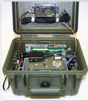
Interior view showing battery and printed circuit board with radio and microprocessor.
