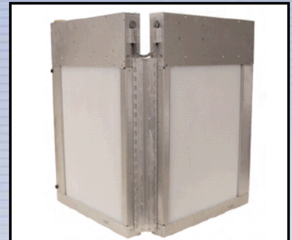
Fission Meter hardware removed from carry bag, showing moderator side.
