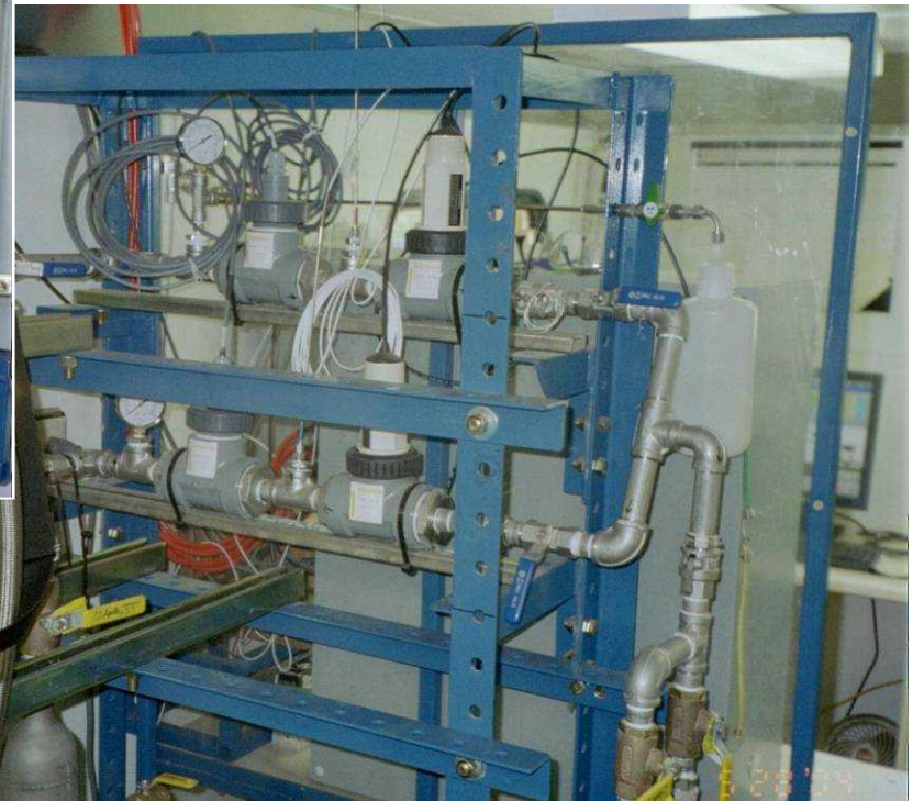
Water Chemistry Inline Measurement Manifold
