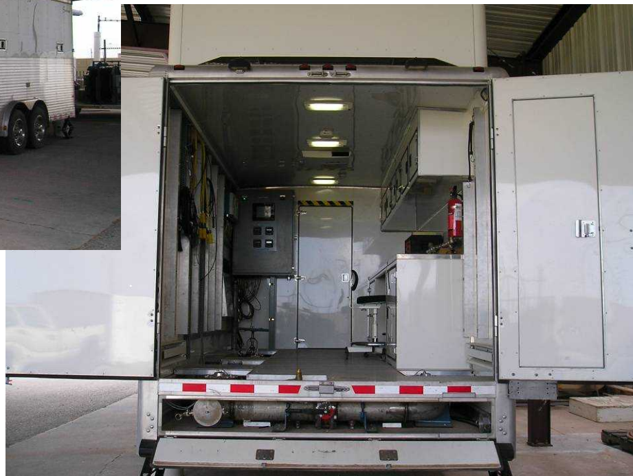
View of Rear Section: DAS Panel, Flowlines, Workbench & Storage Cabinets
