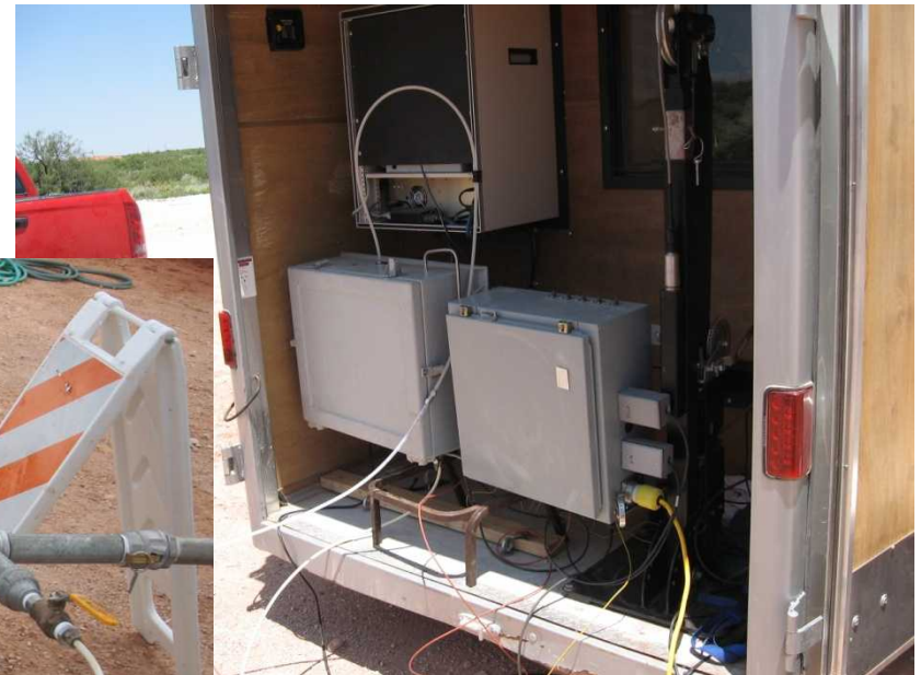
Mini-DAS, WQ Measurement System, and Flowmeters
