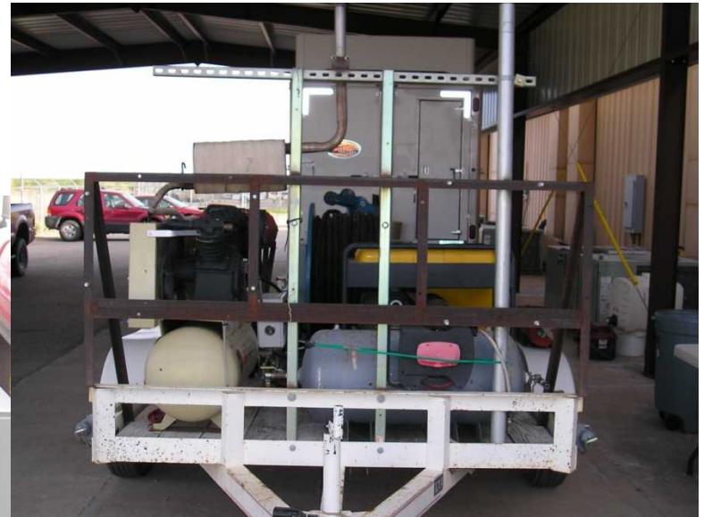
Pump Reel Unit, Generator, & Air Compressor
