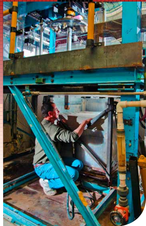
In the top left photo, engineers Pat Brady, left, and Bob McKinnon look over a state-of-the-art drill bit used in deep boreholes. Above, technologist Elton Wright works on a prototype bit used in Sandia's Hard-Rock Drilling Facility. Left, Wright shows a torsional spring used to simulate the rotational vibration of a drill string.
