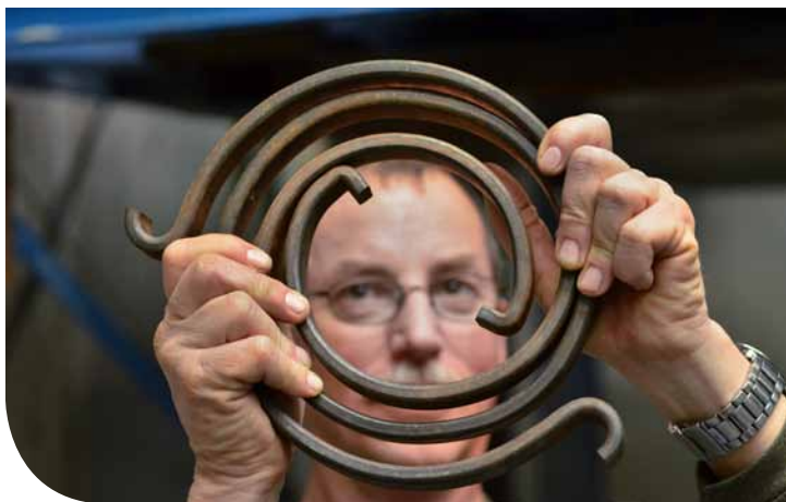
In the top left photo, engineers Pat Brady, left, and Bob McKinnon look over a state-of-the-art drill bit used in deep boreholes. Above, technologist Elton Wright works on a prototype bit used in Sandia's Hard-Rock Drilling Facility. Left, Wright shows a torsional spring used to simulate the rotational vibration of a drill string.
