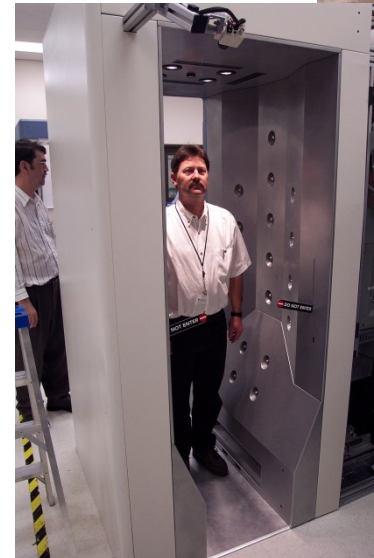
Air nozzles in portal walls “puff” air over subject.
