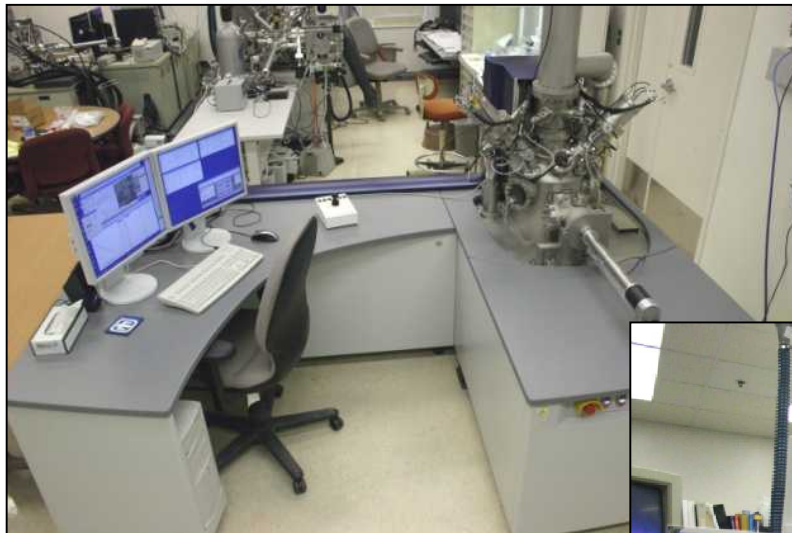
Time-of-Flight Secondary Ion Mass Spectrometry (ToF-SIMS) Tony Ohlhausen
