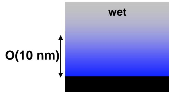
Plasticization,  $\Delta T_g \sim 50^\circ\text{C}$
