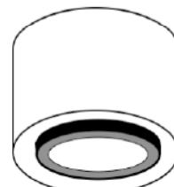
Annulus with I.D. 0.65" and O.D. 0.75" so thickness of 50 mils. Height is also 50 mils
