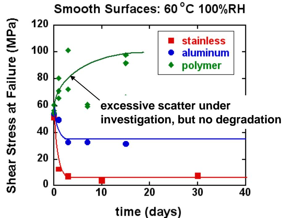
polymer-polymer interfaces (e.g., adhesive to composite) show no degradation
