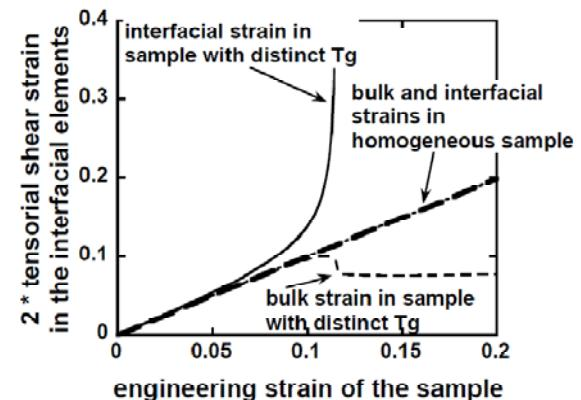
Same failure mechanism, exacerbated by reduced polymer  $T_g$  at interface
