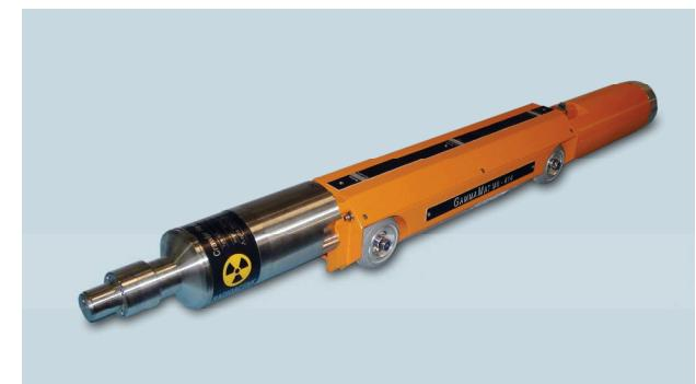
A remotely controlled pipeline crawler. The device drives through the pipe to the proper position, retracts the shielding material to expose film outside the pipe, then moves on to the next weld.
