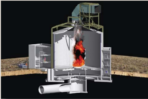
Fire Laboratory for Accreditation of Models by Experimentation/ Radiant Heat (FLAME/RH) in fire mode.
