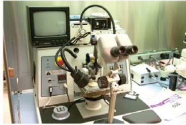
#189A Auto Wedge Bonder - F&K Delvotec 6400
