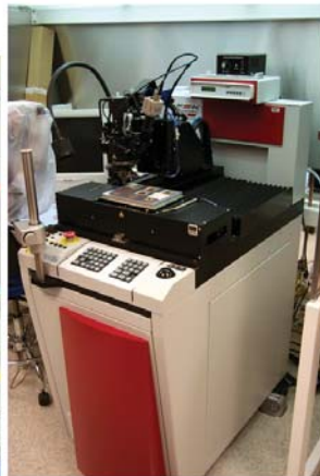
#189A Auto Wedge Bonder - F&K Delvotec 6400
