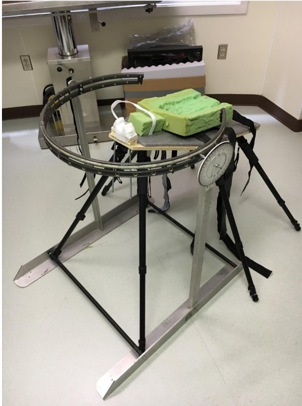
Figure J3. Visual field apparatus and eagle restraint platform fully assembled and ready for an eagle.
