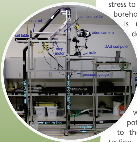
Horizontal and Vertical Erosion Flume
