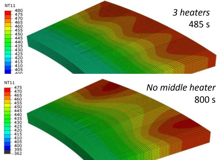
Heat to ~480K, electrical heaters operated at 400 W each
