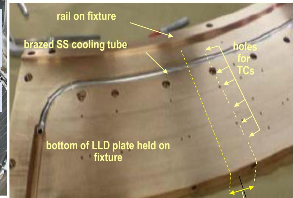
The shape comes directly from the CAD model for fabrication.
