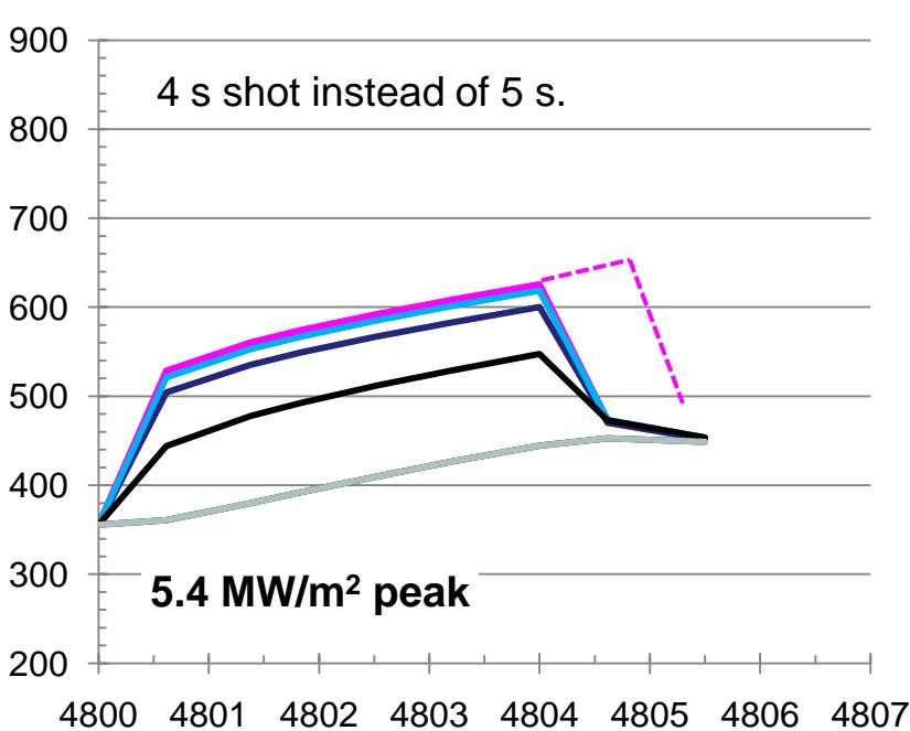
We can confirm that lateral heat conduction accounts for the broadening by comparing the peaked case (above left) to a case with a uniform heat load of 5.4 MW/m<sup>2</sup> over the entire LLD. ( above right).
