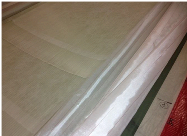
Layers of RodPack before spar cap infusion.
