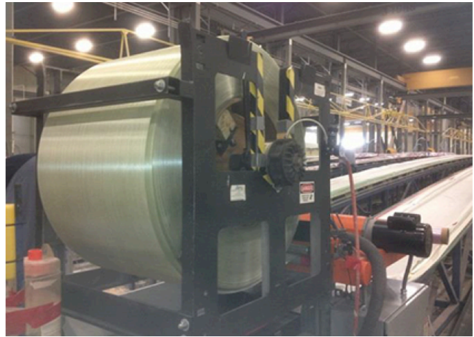
Spool of RodPack spar cap material.
