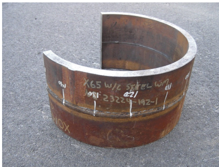
Figure 2. X65 steel girth weld supplied by ExxonMobil.
