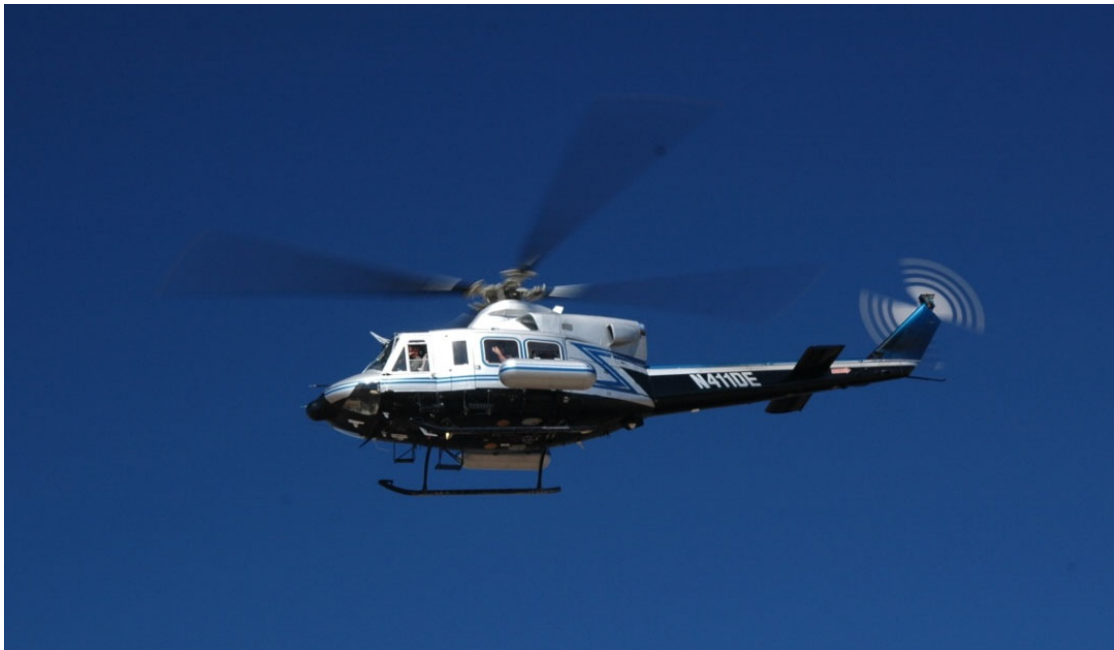
Figure 5. AMS Bell 412 helicopter with externally mounted detector pods.
