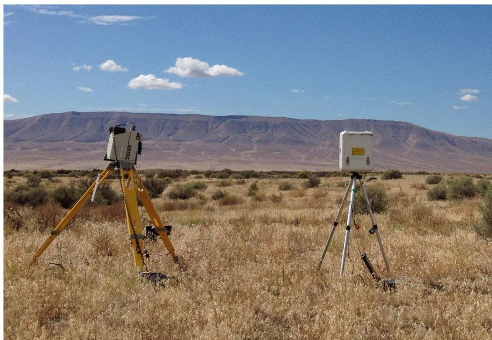
Figure 7. Instrumentation used for ground measurements. The mechanically-cooled high-purity germanium detector is on the left and the pressurized ion chamber is on the right.
