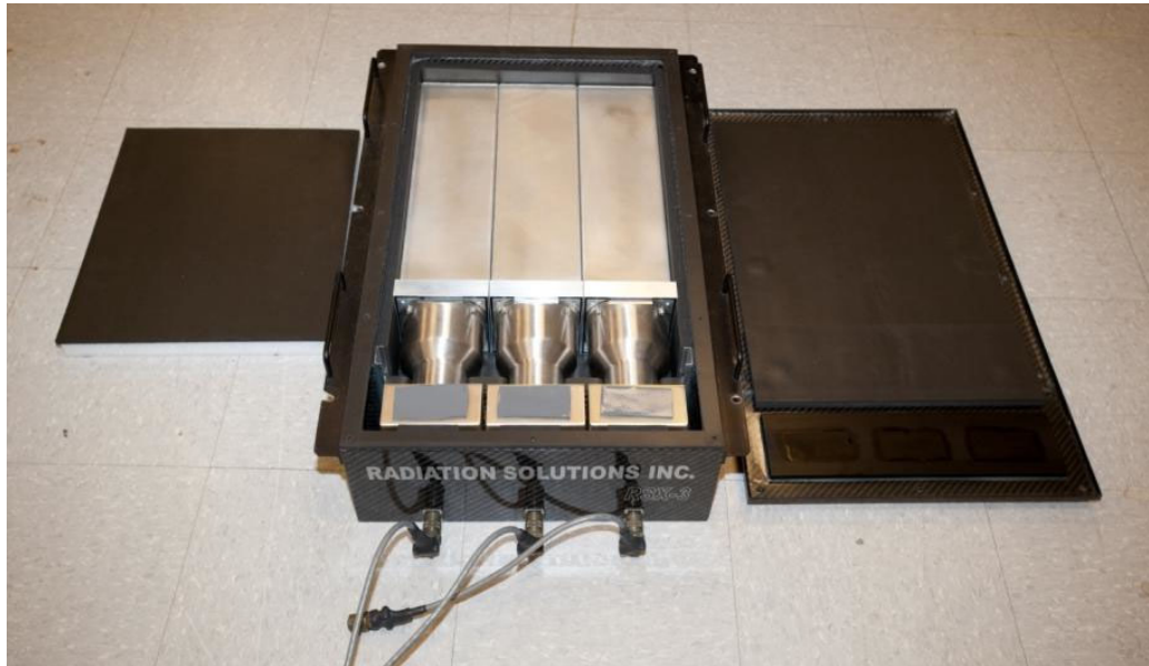
Figure 3. RSX-3 detector. The three 2" × 4" × 16" NaI(Tl) scintillators, three photomultiplier tubes, and three ADS modules can be seen.
