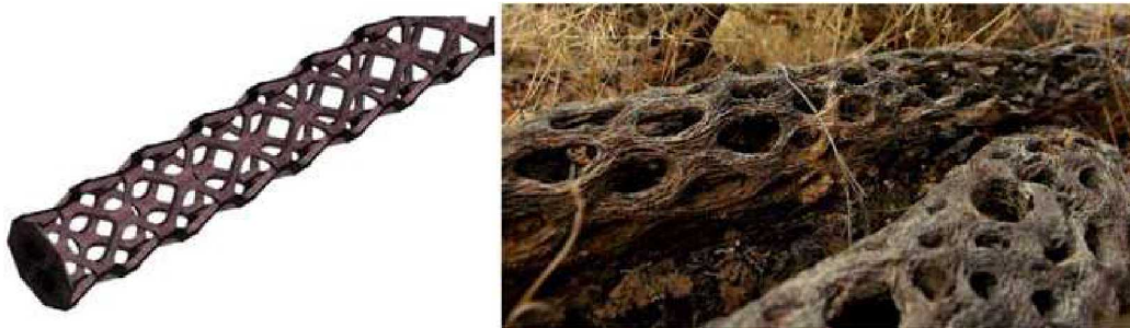
Figure 7.3 Topology optimized bar for a torsion load case (left) [4] that closely resembles the skeletal structure of a cholla cactus (right) [5] . Photo Courtesy: David Gill, Sandia National Laboratories (left); Cholla cactus skeleton image used with permission by Scott Brill at Seekraz.wordpress.com (right).
