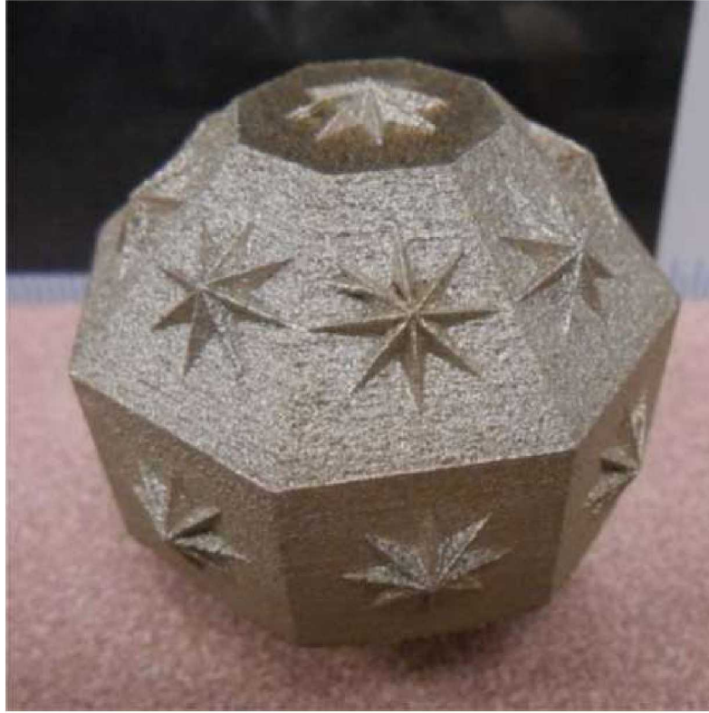
Figure 7.24 A 26-sided, 43 mm wide polyhedron with design features on each face that is relatively easy to print, but much more difficult to measure [78].
