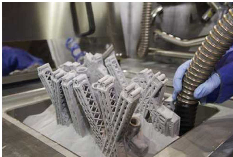
Figure 7.21 Removing the powder surrounding printed parts. Photo Courtesy: APWORKS.
