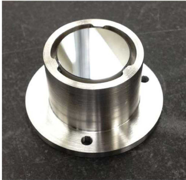
Figure 7.8 An Invar 36 to 304L stainless steel gradient alloy mirror mount. A metal-coated glass mirror is attached to the Invar side of the mount using epoxy. The mirror mount transitions into 304L stainless steel at its base [30,31,32]. Photo Courtesy: NASA Tech Briefs.
