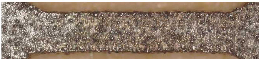
Figure 8.8 As-printed 8 μm S_a rough surface of a 17-4PH stainless steel dogbone with 1 mm gauge width and 4 mm length [20].
