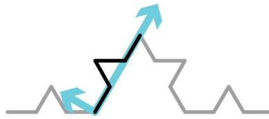
Figure 23.4: Applying the line fractal transform for the Koch Snowflake.
