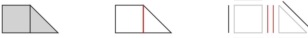
Figure 16.1: Duplicate lines from extracted edges. Consider the small mesh at the left comprising a square and a triangle. If we count the edges in this mesh, we would expect to get 6. However, our naïve implementation in Section 16.1 generates 7 because the shared edge (highlighted in red in the wireframe in the middle) is duplicated. As seen in the exploded view at right, one line is created for the square and one for the triangle.
