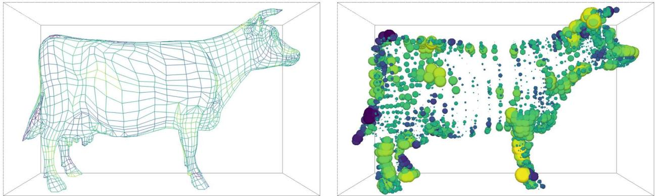
Figure 5.2: Examples of alternate rendering modes using different mappers. The left image is rendered with [MapperWireframe](#). The right image is rendered with [MapperPoint](#).
