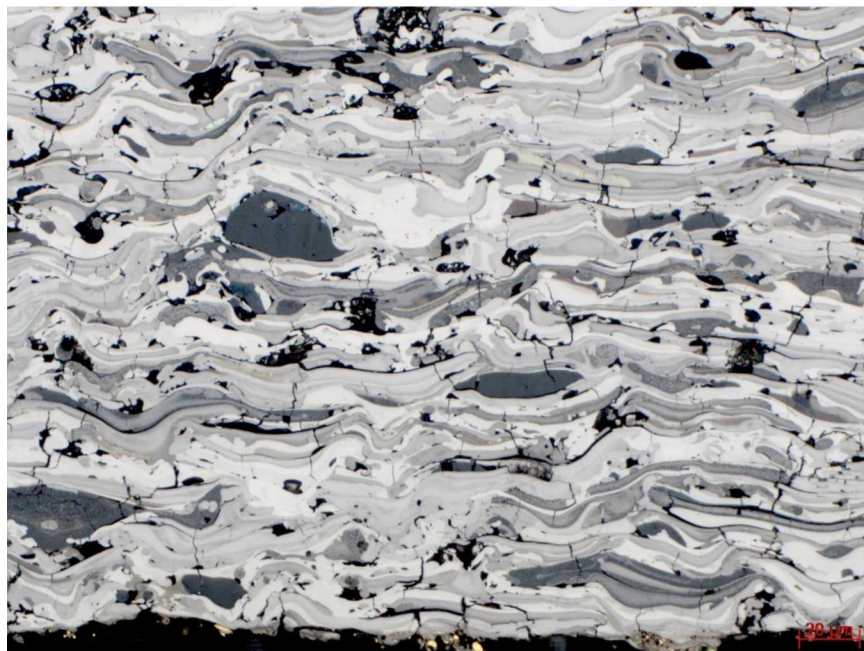
Figure 3-9: 500x magnification image of untested tantalum-niobium sample
