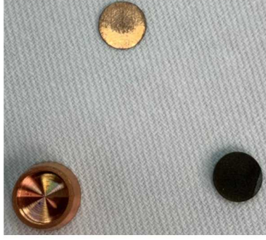
Figure 2-3: Copper cup (left), cap (top) and sample (right) prior to assembly of recovery capsule
