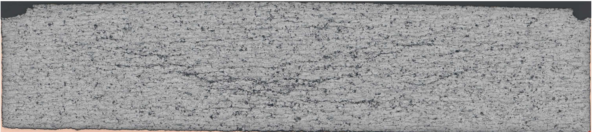
Figure B-2: 200x magnification overview of V543 tantalum sample compressed to 6.3 GPa
