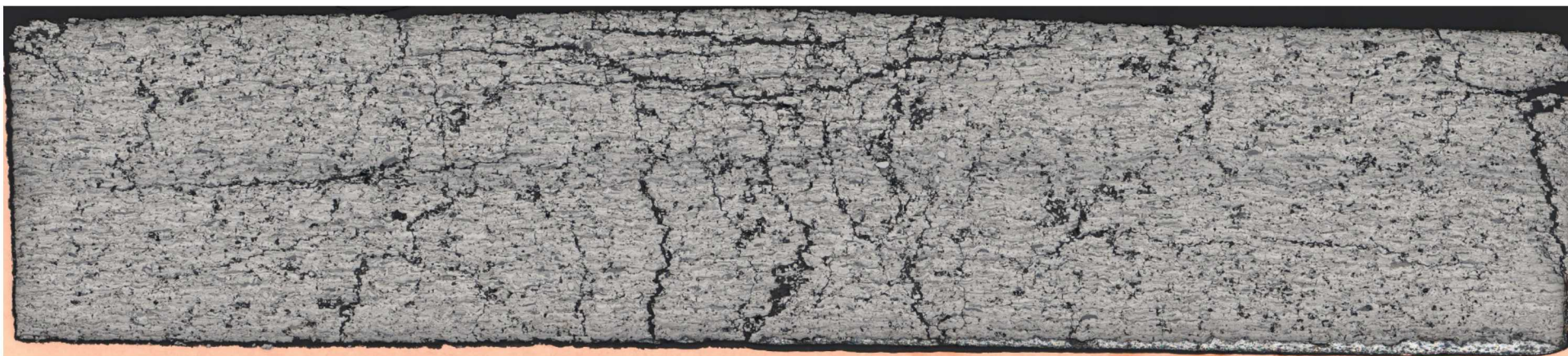
Figure B-6: 200x magnification overview of V546 tantalum-niobium sample compressed to 7.4 GPa
