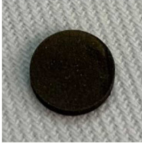
Figure 2-1: Unpolished 5.8 mm diameter sprayed sample
