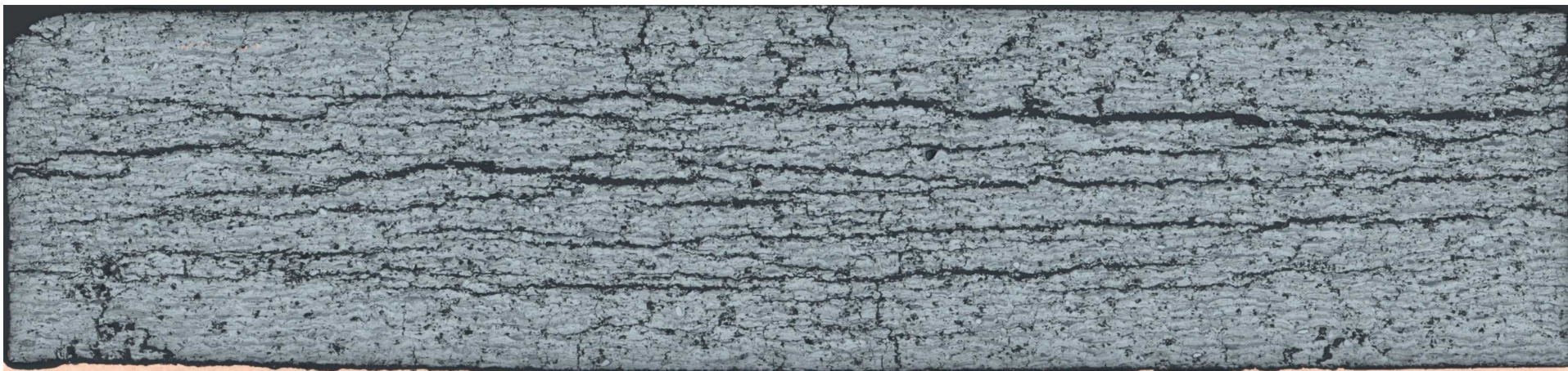
Figure B-5: 200x magnification overview of V544 tantalum-niobium sample compressed to 6.2 GPa
