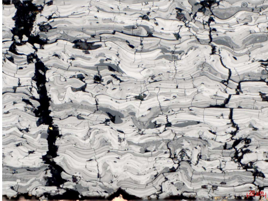
Figure 3-7: 500x magnification image of crack in V545 tantalum sample
