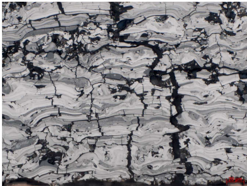
Figure 3-10: 500x magnification image of V544 tantalum-niobium sample compressed to 6.2 GPa
