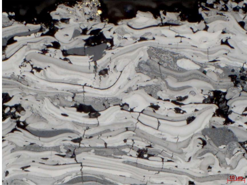
Figure 3-5: 1000x magnification image of untested tantalum sample
