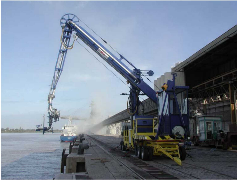
Figure 19 Mobile marine loading arm (Wiese Europe)
