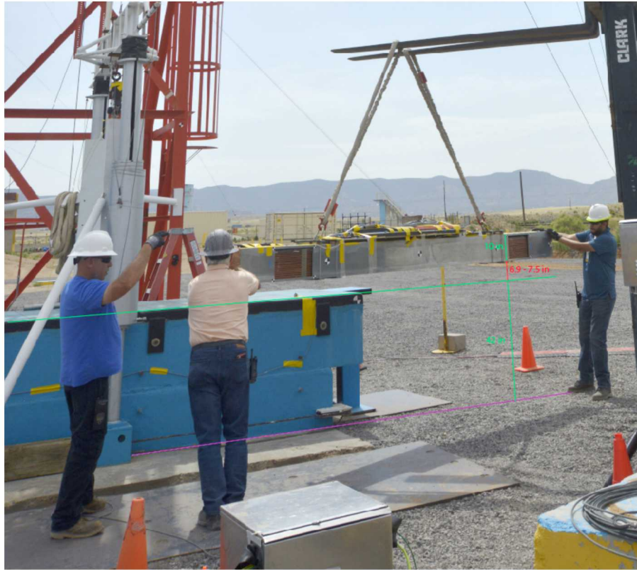
Figure 2-2. Pre-Accident Photo Used in Estimating Accidental Drop Height.
