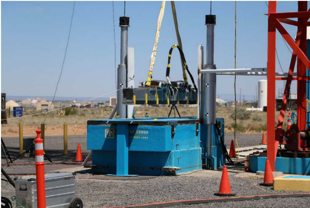
Figure 3-29. Test Unit Seconds before the 30 cm Drop (May 7, 2020, 11:32 am).
