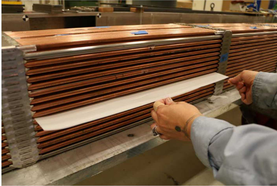
Figure 3-11. Installation of Pressure Paper (2020 Test).
