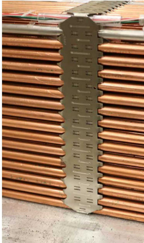
Figure 2-11. Short Span Spacer Grid After 2019 Test.
