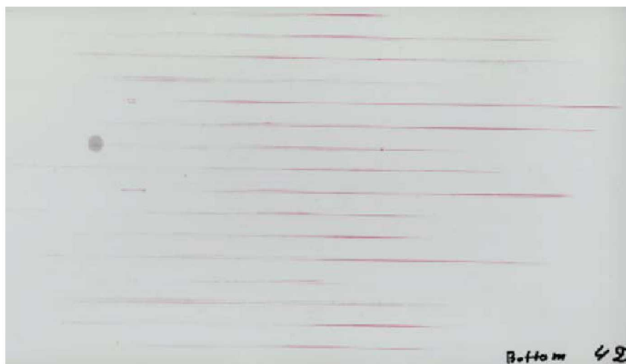
Figure 4-46. Medium Pressure Paper Sheet between the Rods 4 and 5, Assembly Bottom End, Long Span between Spacer Grids (2020 Test).
