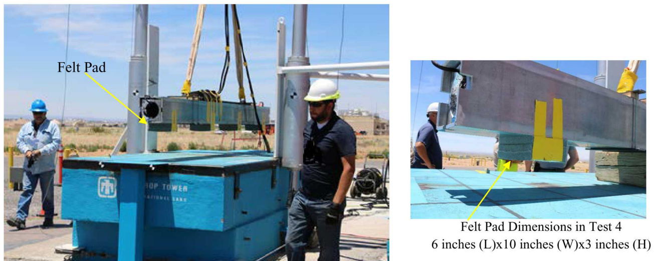
Figure 1-6. Felt Pad Locations (left) and Configuration in Test 4 (right).
