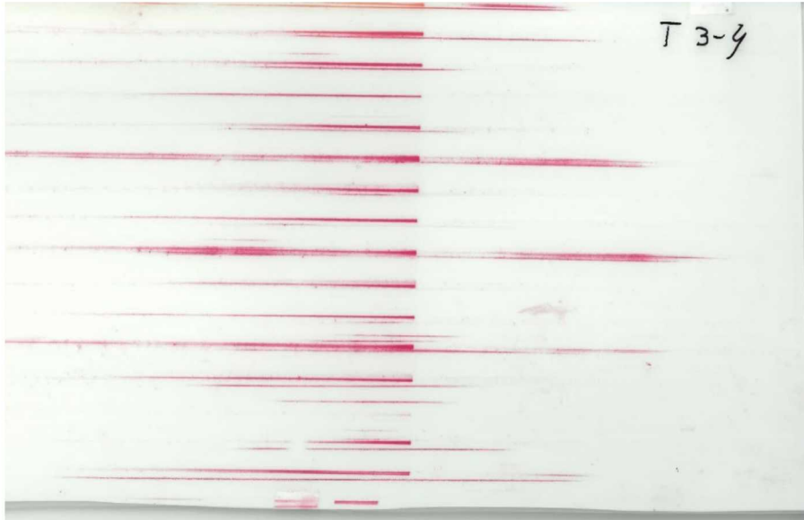
Figure 4-59. Super Low Pressure Paper Sheet between the Rods 3 and 4, Assembly Top End, Long Span between Spacer Grids (2019 Test).
