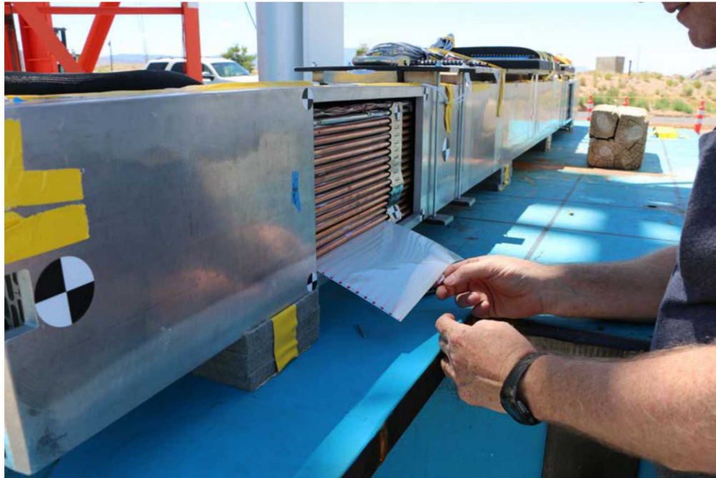
Figure 2-4. Additional Pressure Paper Installed before the 2019 Test.
