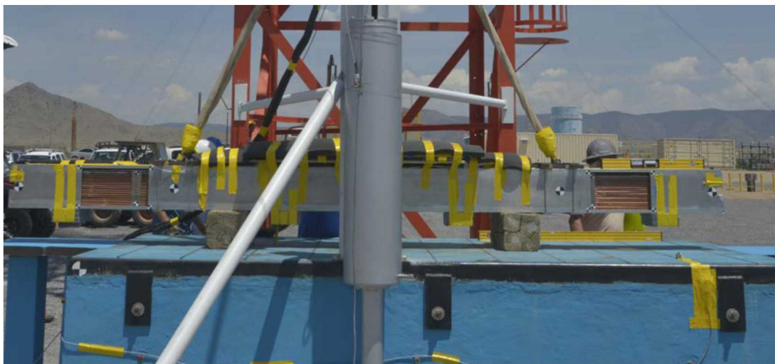
Figure 3-7. Configuration of Felt Pads in 30 cm Drop Test with Damaged Surrogate Assembly (June 2019)
