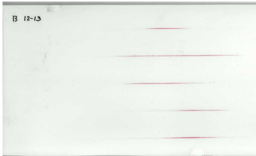
Figure 4-49. Super Low Pressure Paper Sheet between the Rods 12 and 13, Assembly Bottom End, Long Span between Spacer Grids (2019 Test).
