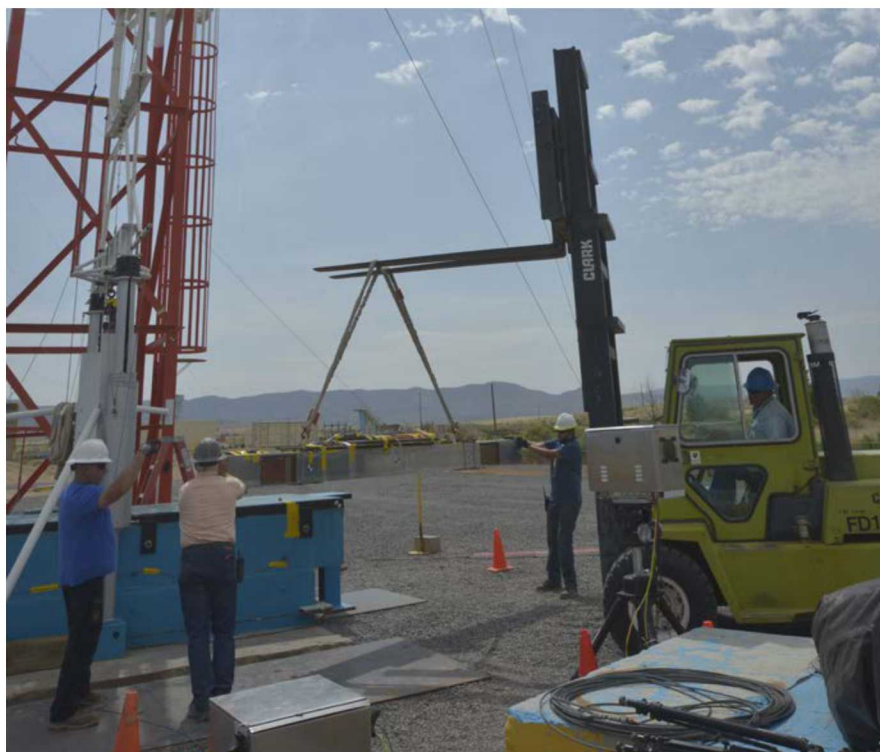
Figure 2-1. Forklift with the Surrogate Assembly Shortly Before the Accidental Drop.
