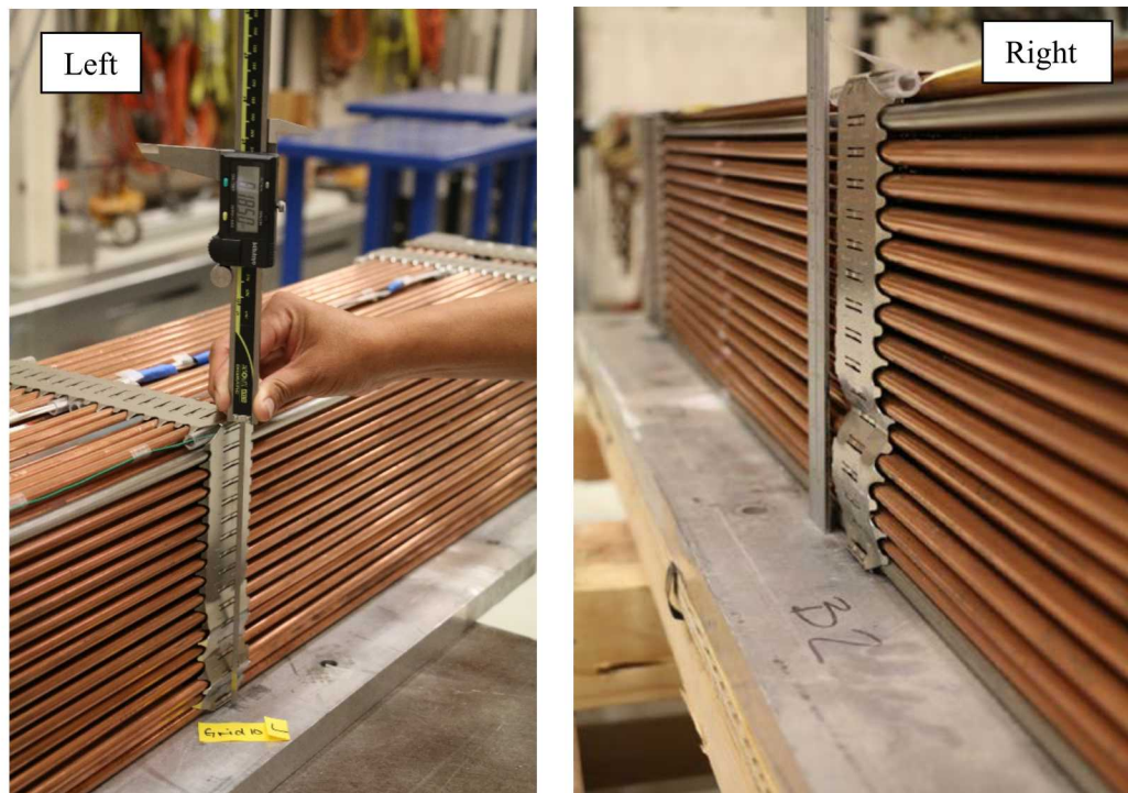
Figure 4-5. Spacer Grid 10 with Largest Deformation in the 2019 Test.
