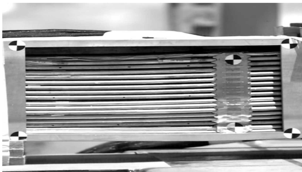
Figure 2-7. Snapshot from the High-Speed Camera Looking at the Basket Tube Window Shortly after the Impact (2019 Test).
