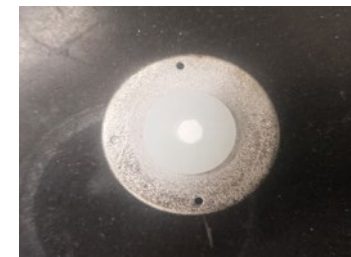
LAZE d_6 -poly(ethylene) target mounted in the catcher
