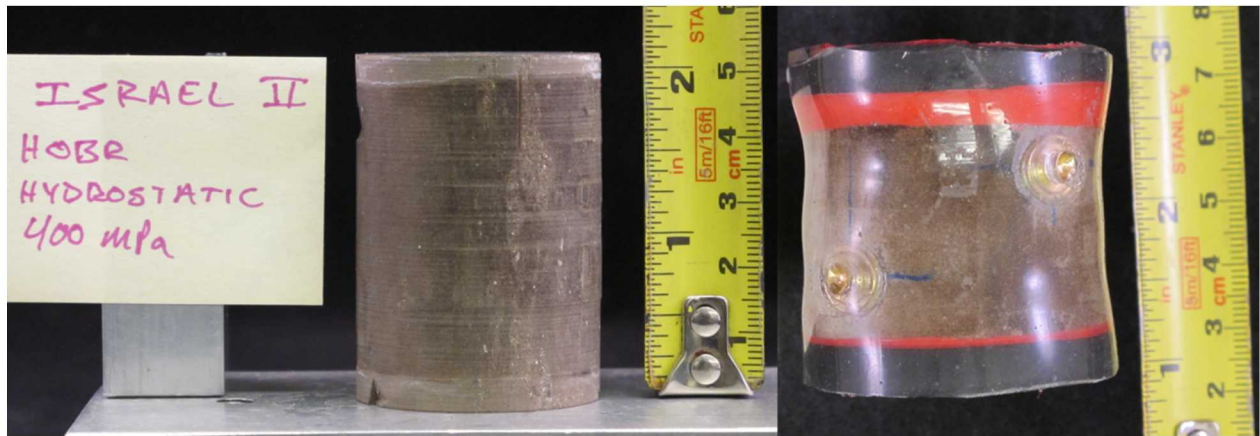
Figure 2 Hydrostatic test sample, note shortening of compacted sample.
