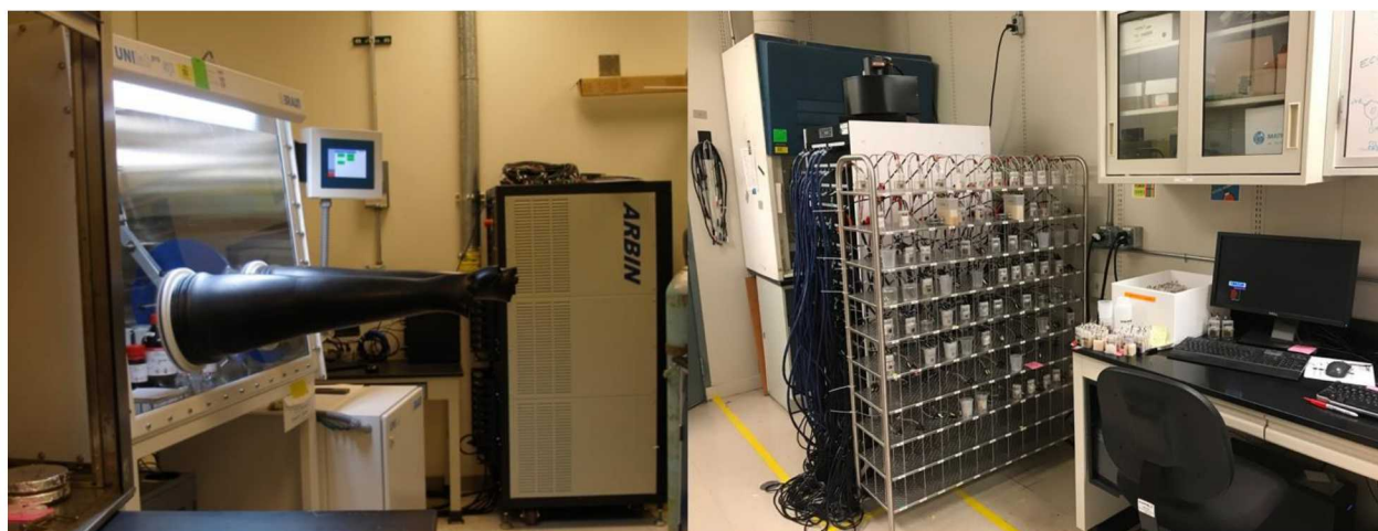
Figure 8. Left: Argon-filled glove box and multichannel battery tester used for laboratory-scale testing of battery performance and reliability. Right: 96-channel battery tester workstation with numerous Zn-MnO 2 batteries undergoing evaluation.
