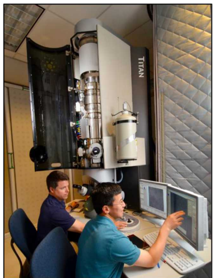
Figure 5. Scientists Paul Kotula and Ping Lu working with the aberration-corrected STEM for atomic scale chemical imaging.
