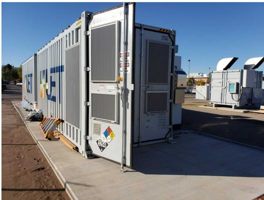
Figure 16. Energy Storage Test Pad (ESTP) at Sandia with a 1 MWh flow battery being tested.
