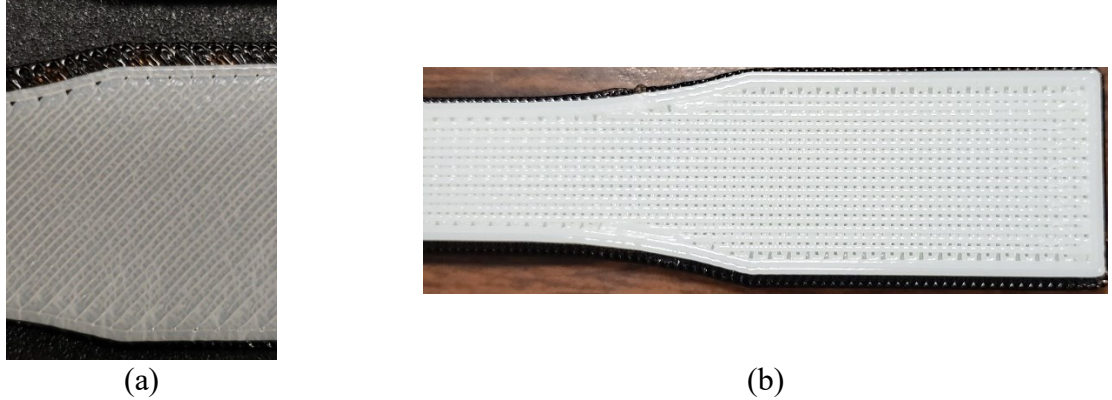
Figure 5. Raster Discretization at Fillet Radius for: (a) ASTM D638 Type I 45°/-45° Raster orientations; and (b) ASTM D638 Type I 0°/90° Raster orientations.
