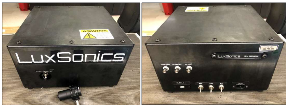
Figure 4. Double differential fiber-optic Sagnac interferometer from LuxSonics, Inc.
