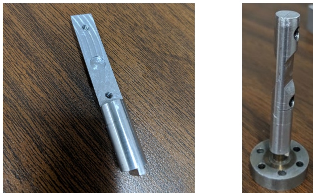
Figure 15: Opened aluminum sample holder with the cavity for the disk of irradiated U-10Zr-1Pd in the thinned section (a). Sample holder closed and attached to the lid of a vanadium can that provides secondary containment of the sample.
