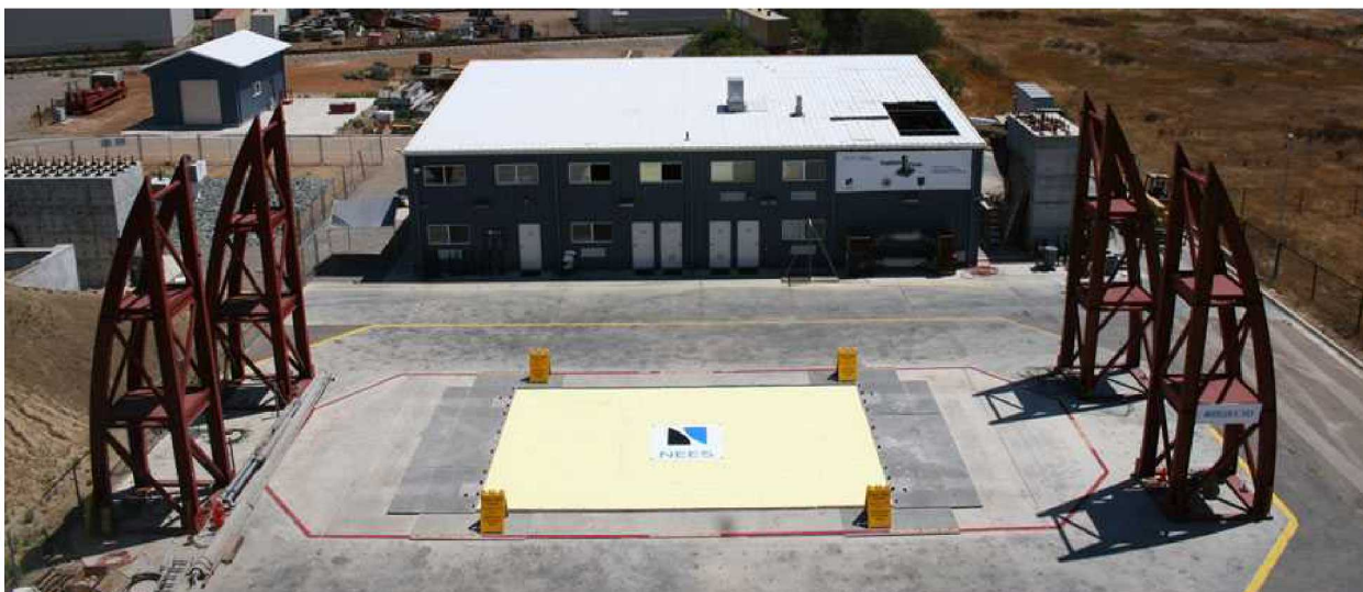
Figure 3-5. NHIERI LHPOST Outdoor Earthquake Simulator (U.C. San Diego) [15].
