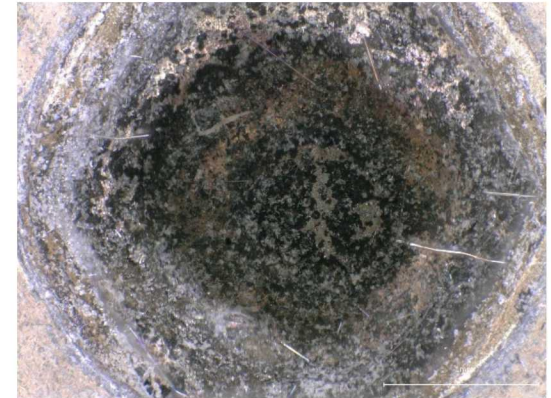
Head of field returned fastener exhibiting numerous whiskers
