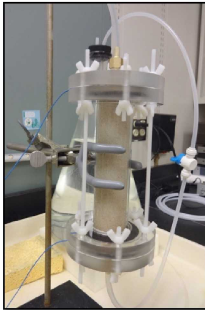
Figure 5-1. Flow-through streaming potential device
