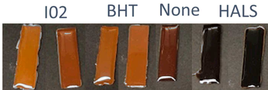
Figure 3. Samples aged at 110^\circ\text{C} for 34 days
