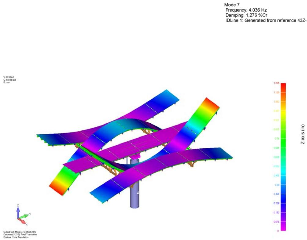
4.036 Hz (note shape 3<sup>rd</sup> mirror module has large motion)
