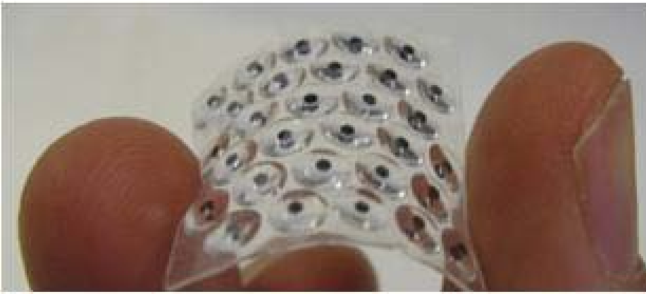
Figure 5 Flexible mechanical model with embedded MEPV cells and micro optics
