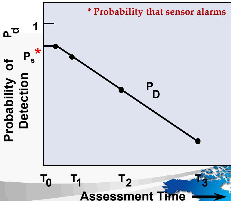
A long time delay between alarm and assessment lowers the probability of detection.
