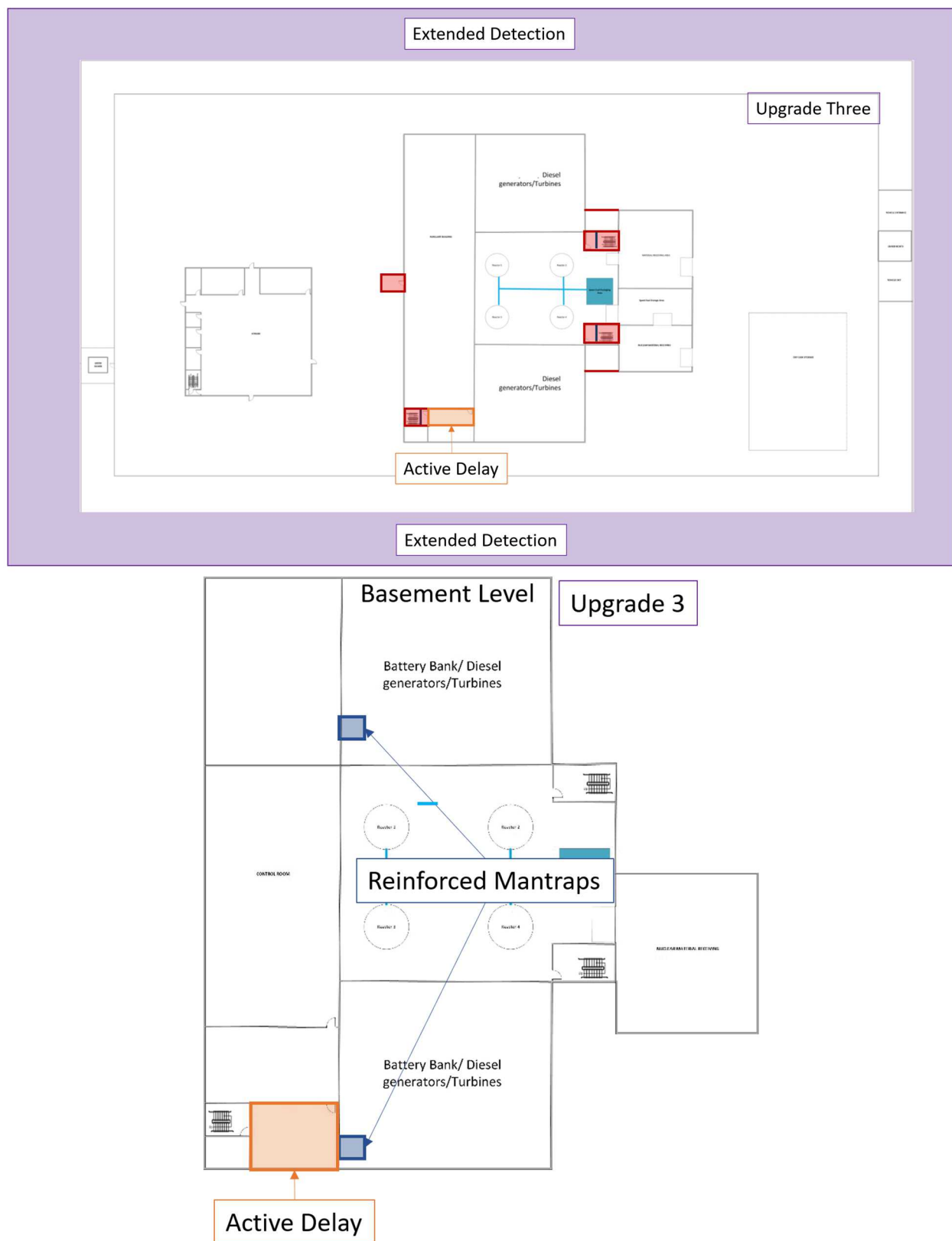
Figure 12. Upgrade 3 - Roll-up Door Active Delay, Extended Detection, Active delay along the battery bank path
