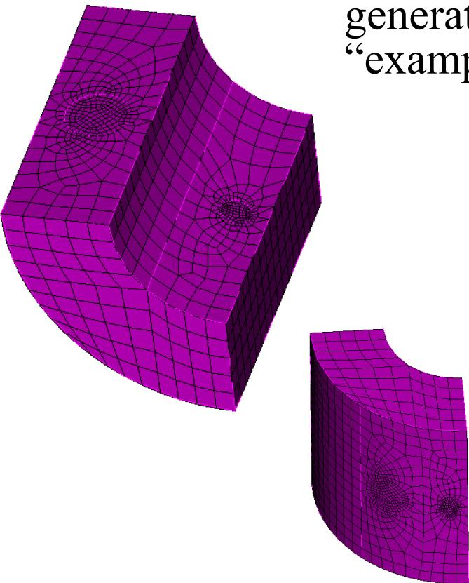
Manually set vertex types to generate the mesh on the left for “example2.cub”.
