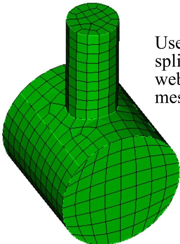
Use only curve splits, surface splits, and setting vertex types (no webcutting!) to generate a hex mesh for “example3.cub”.
