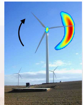
Measurement of blade trailing edge noise (S. Oerlemans, Ph.D. Thesis, U. of Twente, 2009)
