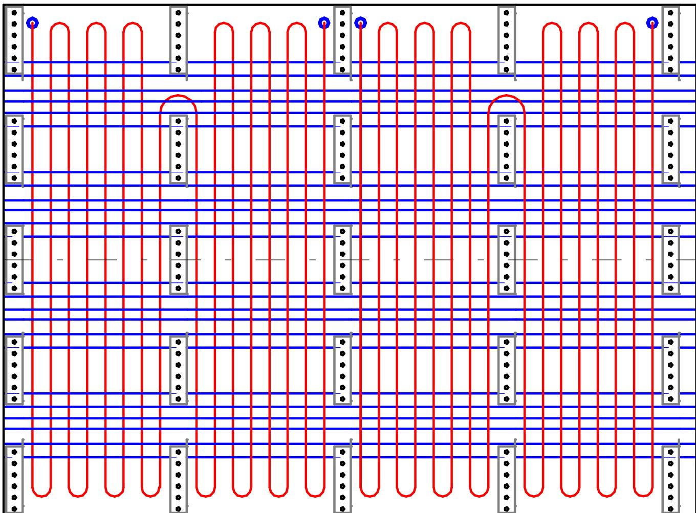
The entire length of each fiber will be interrogated by measuring Rayleigh backscatter. Methods and layouts to bond the sensor to the other panel are currently being explored.
