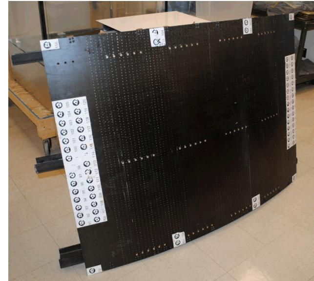
Image: Full-scale carbon fiber aircraft fuselage section with co-cured stringers and attached frames, **similar to the ones that are currently being fabricated** for impact testing.
