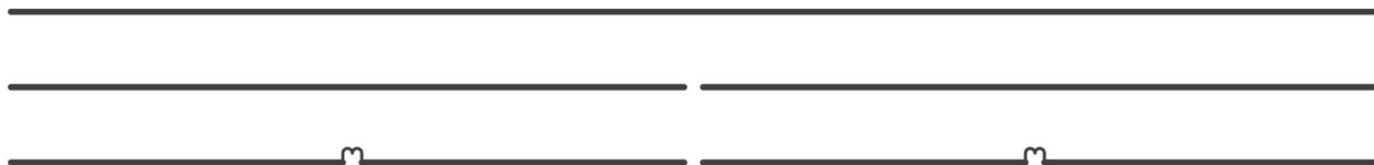
Figure 2-16. Simulated cable configurations (from top to bottom): solid cable, split cable (one spark gap), and split cable with each half loaded with an inductor in the center.
