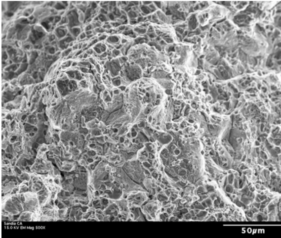
Air induced fracture of sample B201, 2618 Al, at 500x
