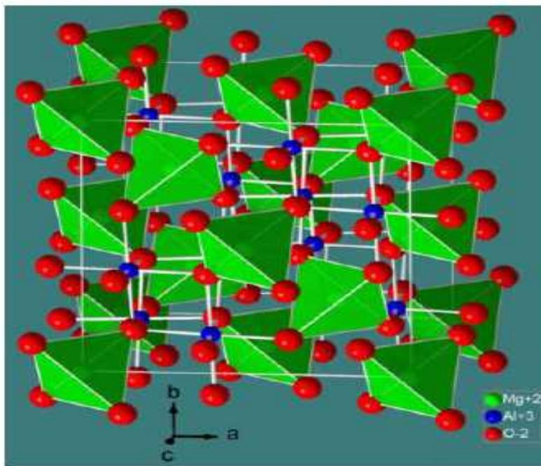
To the left is the spinel oxide unit cell. The red atoms are oxygen, while the green atoms occupy the tetrahedral sites and the blue atoms occupy the octahedral sites.
