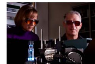
Photoluminescence (PL) lifetime measurement: Researchers measure the PL lifetime of a quantum dot solution. We are developing these materials as red-emitters for SSL, in an effort to produce highly efficient light sources with good color rendering.
