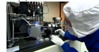
Evaluating Efficiency: Emission from a green light-emitting diode (LED) test structure fabricated at Sandia National Laboratories. Understanding efficiency limitations of InGaN LEDs is a major thrust of our EFRC.
