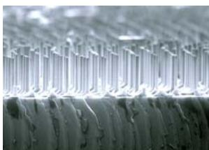
Nanowire-based LEDs: SEM of an ordered gallium nitride (GaN) nanowire array fabricated on sapphire wafers by a two-step etching process. GaN-based nanowires may be used to create higher performance LEDs in the future due to their unique properties.
