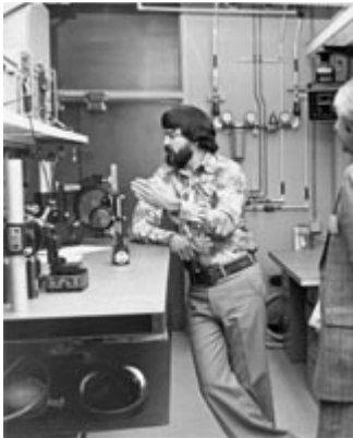
Pete Witze describes his Schlieren system for imaging flame propagation in a spark ignition engine.
