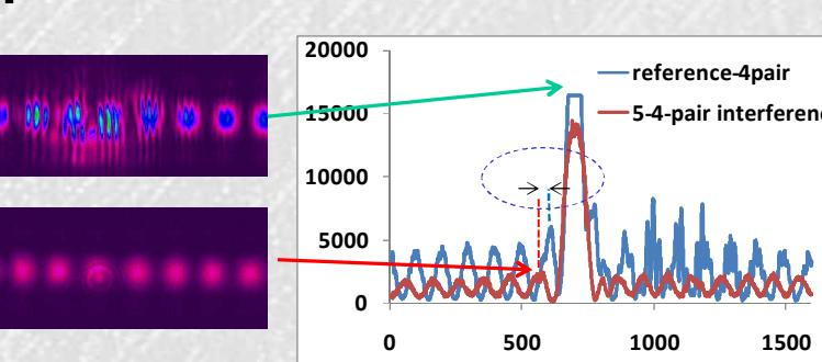
An additional phase shift is introduced for the electromagnetic wave traveling through the slit containing 5 pairs of multilayers versus 4, resulting in a shift in the interference fringes ( shown in red above) compared to the case when both slits have 4pairs (blue) .
