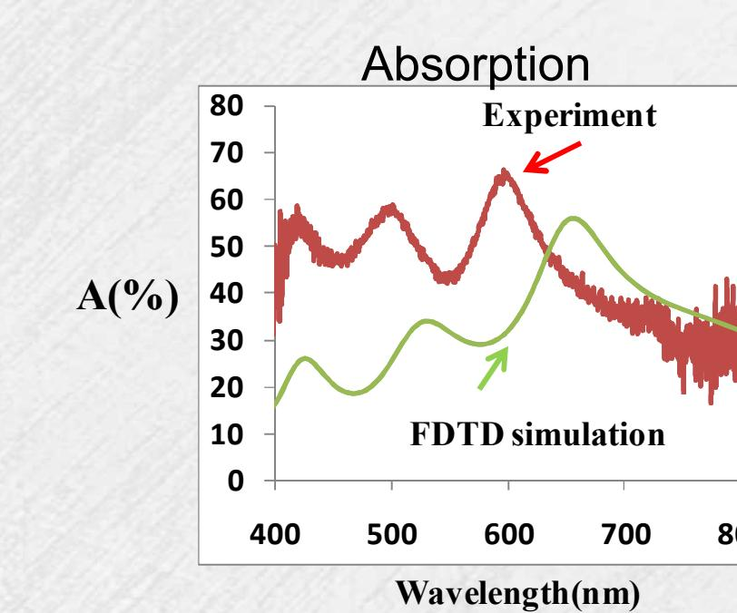
The wavelength at which the fabricated multilayer composite structure displays ENZ behavior can be experimentally determined by performing Young's double slit type experiment which measures the amplitude and the phase difference between ENZ composite structure of different thickness deposited on each slit. Since the multilayer structures are highly anisotropic this approach enables near normal incidence measurements unlike ellipsometry, which is done at large angles.
