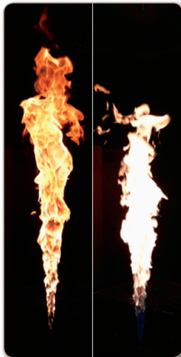
Figure 2. Photographs of JP-8 surrogate jet flame (left) and ethylene jet flame (right), both with a fuel jet Reynolds number of 20,000.
