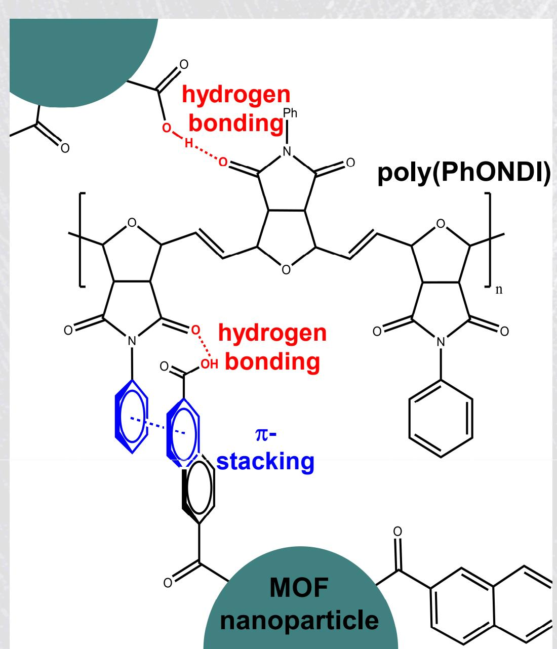
The poor breakdown performance of composites is often attributed to poor compatibility between the polymer and the inorganic filler, leading to poor dispersion and integration. We propose that metal-organic frameworks, which have intrinsic organic functionality, used as the filler in a MOF/polymer composite, may provide improved compatibility and dispersion, and yield composites with improved properties relative to traditional inorganic/polymer composites.
