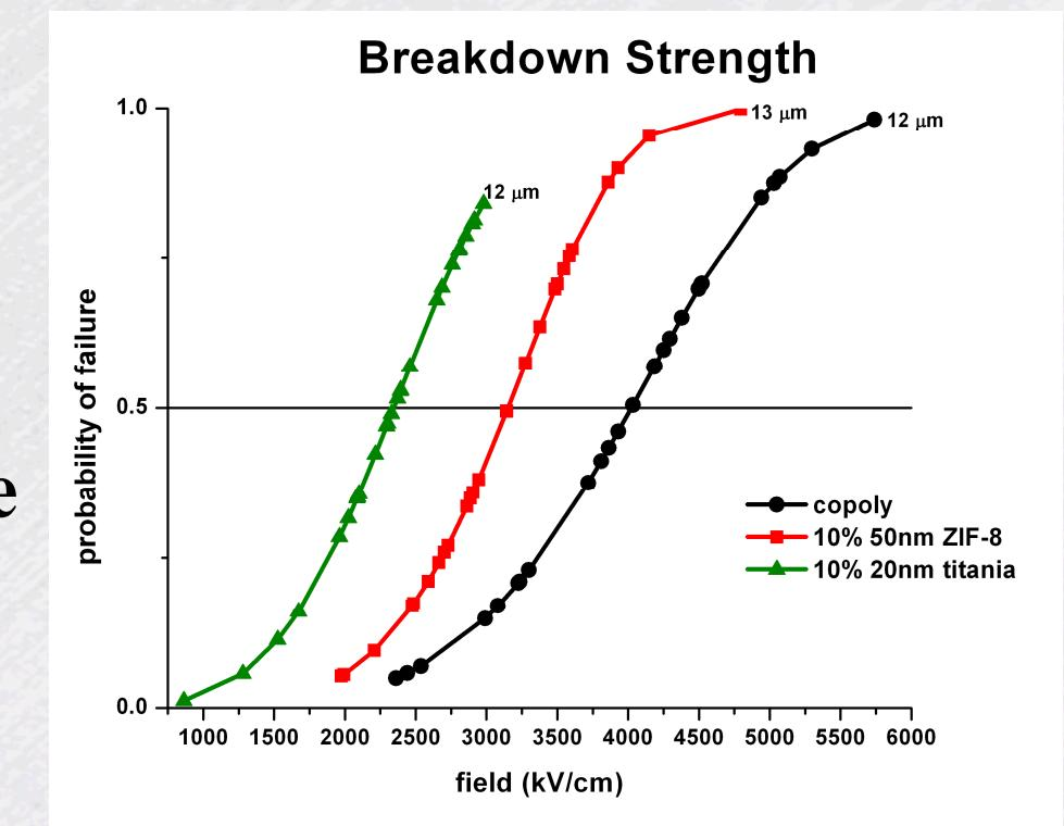
Although the ZIF-8 composite outperforms the  $\text{TiO}_2$  composite, due to the lower breakdown strength relative to the polymer alone, the energy density of the composite does not improve relative to the polymer.
