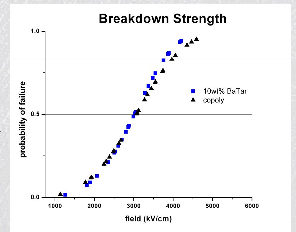
High breakdown strength is maintained, however, the small change in permittivity results in minimal improvements in energy density.
